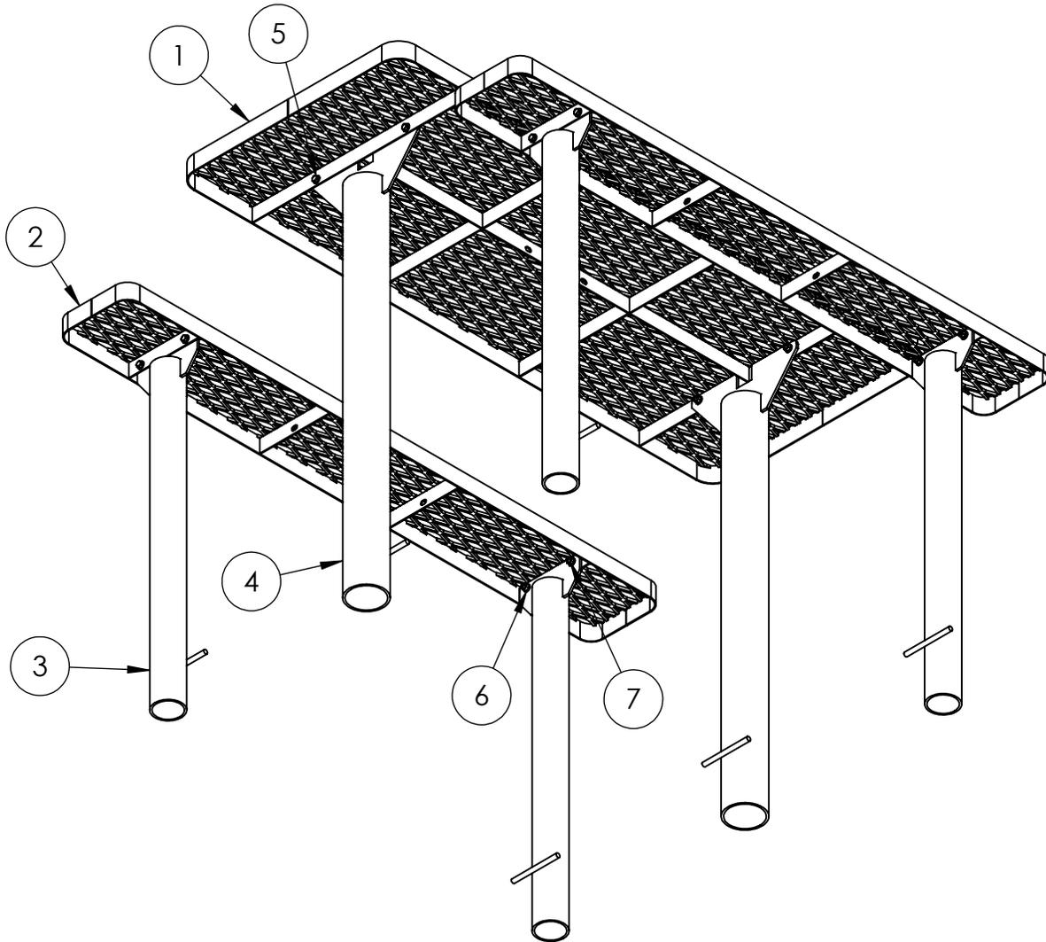
1. Drill 6 holes in the ground per the drawing on page 1.
